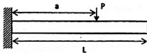
A cantilever beam of length L and uniform flexural rigidity EI is subjected to a transverse load P at a distance 'a' from the fixed end as shown in the figure. The deflection of the beam at the free end would be
