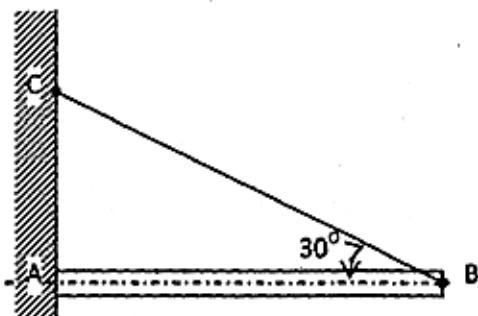
A uniform bar AB (figure) weighing 100 kg is hinged at A to a vertical wall and held in a horizontal position by a cord BC. Tension in the cord BC will be
