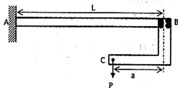
A cantilever beam AB of length L and uniform flexural rigidity EI has a rigid bracket BC attached to its free end as shown in the figure. End C is subjected to a vertically downward force P. If deflection at point B is zero, then  $\frac{a}{L}$  should be
