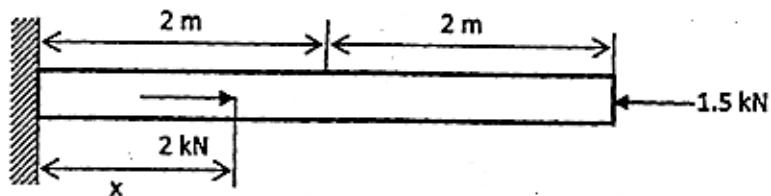
A prismatic steel bar having cross-sectional area  $3 \text{ cm}^2$  is subjected to axial forces as shown in the figure. Young's modulus of the material of the bar is 200 GPa. Load 2kN acts at a distance  $x$  from the left fixed end of the bar. For no change in the length of the bar,  $x$  will be
