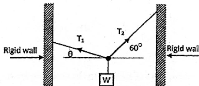
A weight  $W$  is supported by two cables as shown in the figure. Tension  $T_1$  of the left cable will be minimum when value of  $\theta$  is
