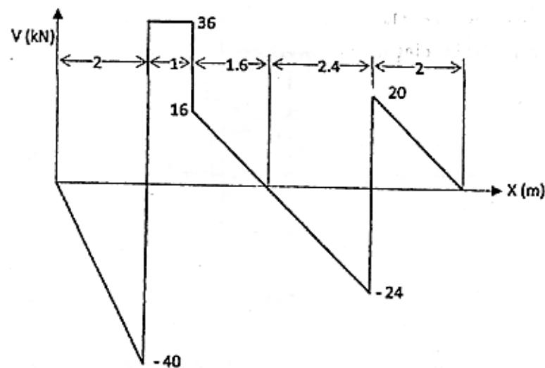
Shear force diagram of a beam is shown in the figure.
