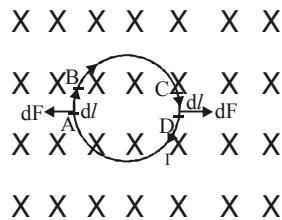
On element CD, the direction of force will be towards right on the plane of the paper and the magnitude will be  $dF = IdlB$ .
