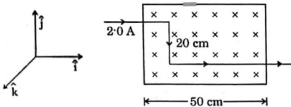
**Solution: Concept:** Force on a current-carrying straight conductor:
