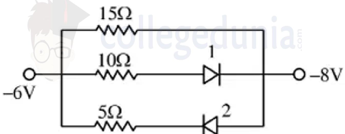
Diode 2 is in reverse bias, so no current will flow through the branch containing it. It can be treated as a broken wire.
