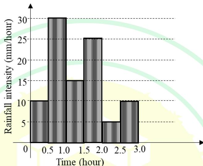
If the storm produced a direct runoff of 12.5 mm, then the  $\phi$ -index of the storm for the catchment is \_\_\_\_\_ mm/hour. (rounded off to two decimal places)
