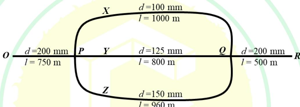
Diameter ( $d$ ) and length ( $l$ ) of each pipe are as presented in figure and all pipes are of same material having friction factor ( $f$ ) of 0.02. Assume acceleration due to gravity ( $g$ ) as  $10.0 \text{ m/s}^2$ . If the head difference between **P** and **Q** is 10 m, then the head loss between **Q** and **R** is \_\_\_\_\_ m. (rounded off to two decimal places)
