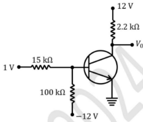
The value of common-emitter current gain  $\beta$  for the transistor is 100. Ignore reverse saturation current. The output voltage  $V_0$  (in V) is \_\_\_\_ (in integer).
