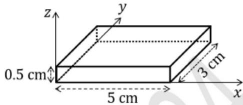
When the majority charge carrier concentration is  $12.5 \times 10^{13} \text{ cm}^{-3}$  and the sample is exposed to a constant magnetic field applied along the  $+z$ -direction, a Hall voltage of 20 mV is measured with the negative polarity at  $y = 0$  plane. Take the electric charge as  $1.6 \times 10^{-19} \text{ C}$ . The concentration of minority charge carrier is negligible. Which of the following statement is/are true?
