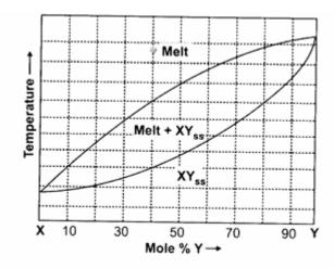
Which of the following statements is/are correct for crystallization of a starting melt of composition XY (the dot in the diagram)?
