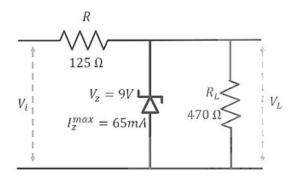
(A)  $V_{\min} = 9.0 V$  and  $V_{\max} = 11.4 V$
