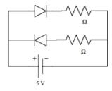
Given: each diode drop =  $0.7 \,\mathrm{V}$ , battery =  $5 \,\mathrm{V}$ , resistors =  $1 \,\mathrm{k}\Omega$ .
