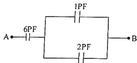
Determine the equivalent capacitance between the points A and B in the adjoining figure.
