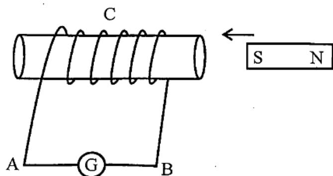
A magnet is brought towards a coil as shown in the adjoining figure. In which direction the induced current will be?
