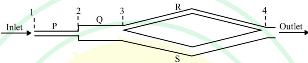
(A)  $\Delta h = h_P + h_Q + h_R + h_S$  and  $V_P d_P^2 = V_Q d_Q^2 = V_R d_R^2 = V_S d_S^2$
