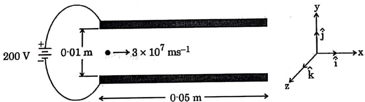
A pair of square conducting plates having sides of length 0.05 m are arranged parallel to each other in x-y plane. They are 0.01 m apart along z-axis and are connected to a 200 V power supply as shown in the figure. An electron enters with a speed of  $3 \times 10^7 \text{ ms}^{-1}$  horizontally and symmetrically in the space between the two plates. Neglect the effect of gravity on the electron.
