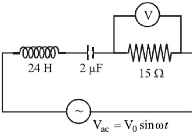
The frequency, at which the voltage across the resistor is maximum, is :
