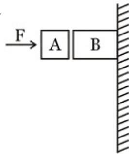
Given in the figure are two blocks  $A$  and  $B$  of weight 20 N and 100 N, respectively. These are being pressed against a wall by a force  $F$  and kept in equilibrium as shown. If the coefficient of friction between the blocks is 0.1 and between block  $B$  and the wall is 0.15, the frictional force applied by the wall on block  $B$  is:
