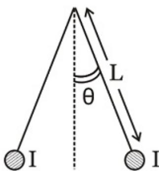
Two long currents carrying thin wires, both with current  $I$ , are held by insulating threads of length  $L$  and are in equilibrium as shown in the figure, with threads making an angle '  $\theta$  ' with the vertical. If wires have a mass  $\lambda$  per unit length then the value of  $I$  is:
