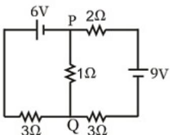
In the circuit shown, the current in the  $1\ \Omega$  resistor is:
