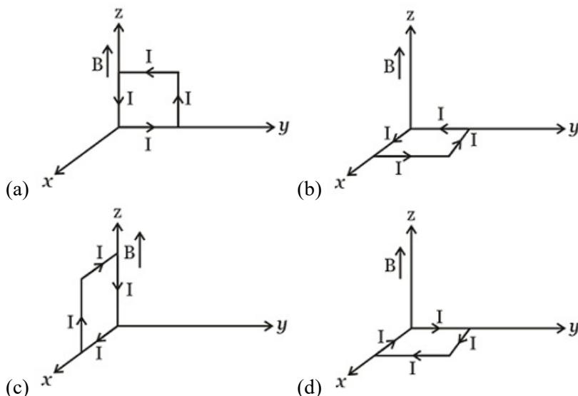
If there is a uniform magnetic field of 0.3 T in the positive  $z$  direction, in which orientations the loop would be in (i) stable equilibrium and (ii) unstable equilibrium?
