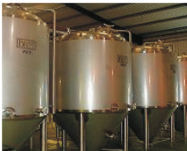
Fig. 8.4 (NCERT): Industrial fermentors — large stainless-steel vessels where microbes are cultured in carefully controlled conditions (temperature, pH, dissolved oxygen, mixing speed) to produce commercial quantities of beverages, antibiotics, enzymes or organic acids.
