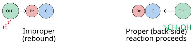
Fig. 7: Effective collisions require correct orientation. Left: \text{OH}^- approaching the Br side simply rebounds. Right: back-side attack on the carbon leads to product. The steric factor P captures the orientation probability.
