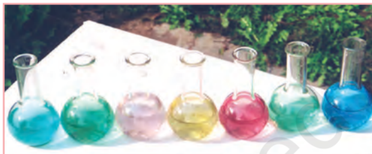
Fig. 4.5: Colours of some of the first row transition metal ions in aqueous solutions. From left to right: \text{V}^{4+} , \text{V}^{3+} , \text{Mn}^{2+} , \text{Fe}^{3+} , \text{Co}^{2+} , \text{Ni}^{2+} and \text{Cu}^{2+} .
